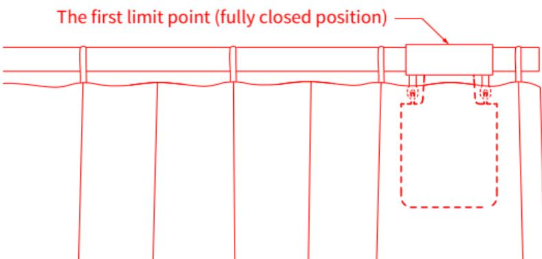
C) Meanwhile, the Curtain Driver will automatically run to the opening limited point and stop after being pulled in the fully opening direction for about 10cm. After the long "beep", another limit point is automatically and successfully set, which means the opening range of the device is set up.
