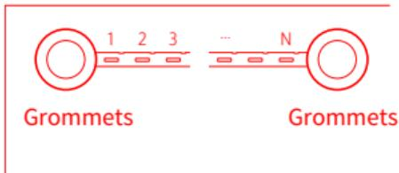
2. Install the first clip onto the third hole from the left of the rubber strip, and install all the other clips according to the following instructions.
