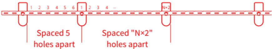
3. Please install the rubber strip together with the clips on the curtain according to your curtain layout as shown below.
