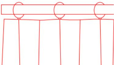
If you are using grommet curtains, the minimum spacing between two grommets should be greater than 95mm.
