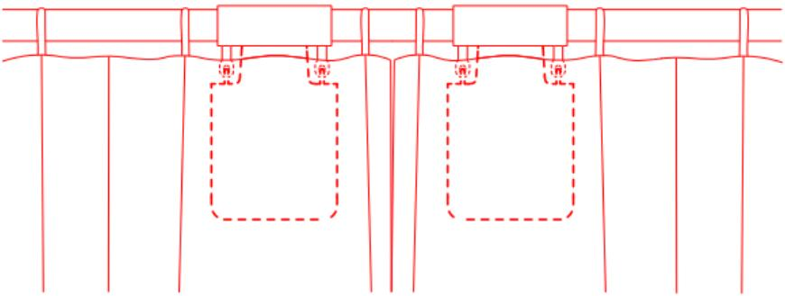
B) Set the opening distance for Curtain Drivers on left and right sides according to Step B and C for that of "single-sided curtains".
